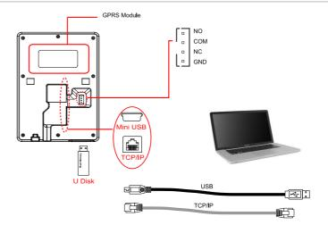
★ SIM Installation (Please power off the device to installation the SIM Card.)
