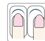
Finger not placed on the center of the sensor.
