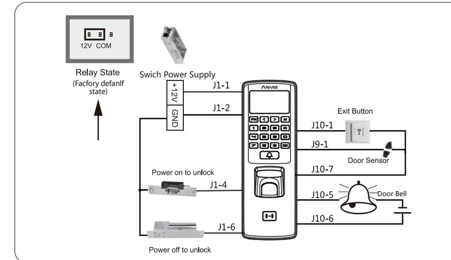
The following wiring is recommended to prevent damage to the device when load is large.
