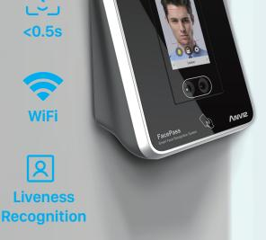
FacePass 7 facial recognition terminal is equipped with AI deep learning Architecture and infrared live detection technology, which can achieve 24/7 accurate identification for virous environment conditions and can effectively prevent fake faces such as photos and videos.
