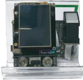
Face all in one module not only face verification also include fingerprint, RFID and Password verification. It is adopts Embedded Linux System and Anviz the latest hardware platform. The face all in one module can be wide range of products such as Time attendance and Access Control Device.
