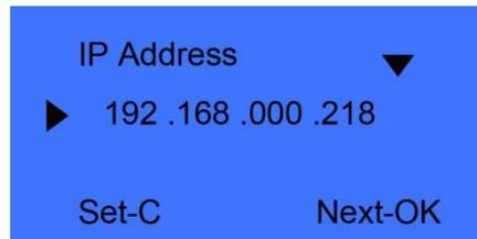
Press [◀ IN] or [OUT ▶] key or number key to input IP address. Press [OK] key to shift between the 4 segments. After set is completed, press [C] key to enter IP address save interface.
