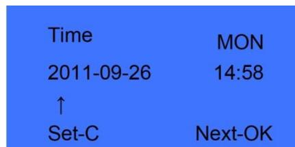
You can press the [OK] key to move the cursor to shift the year, month, day. And use number and [◀ IN] or [OUT ▶] key adjust the time. After setting completed, press [C] key and enter system time save interface.
