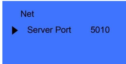
Press [◀ IN] or [OUT ▶] key or number key to input server port. After set is completed, press [C] key to enter save interface.
