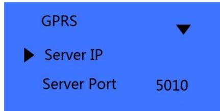
Server IP: The server IP is the Public IP address (it is from ISP). It is the PC Server IP that the T60/TC530 device will connected with.
