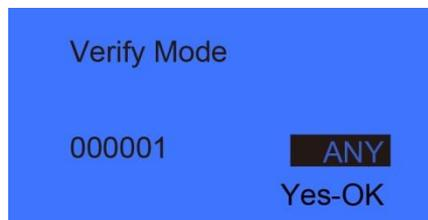
Setting employee's verify mode through [◀ IN] or [OUT ▶] key, then press [OK] key to confirm and enter save interface:
