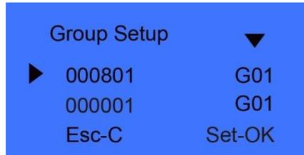
Press [◀ IN] or [OUT ▶] key to select user ID or press [OK] to input user ID manually.
