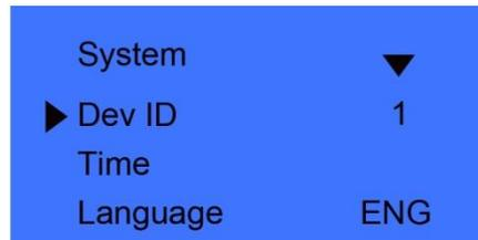
**Note:** Device ID range is 0-99999999, and default is 1.(Device ID must enter as same as in the communication software), When the device as “0”, must use the lasted 8 digit of the serial number to communication with software.
