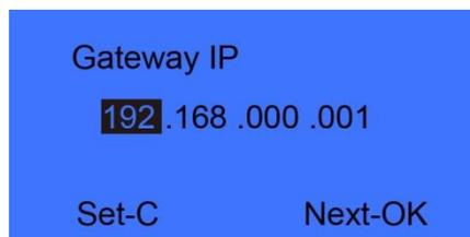
Press [◀ IN] or [OUT ▶] key or number key to input gateway IP. Press [OK] key to shift between the 4 segments. After set is completed, press [C] key to enter gateway IP save interface.
