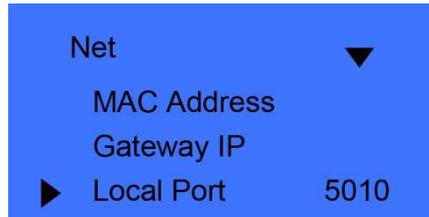
Press [◀ IN] or [OUT ▶] key or number key to input port. After set is completed, press [C] key to enter save interface.
