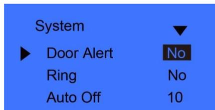
Press [◀ IN] or [OUT ▶] key or number key to input door alert value. Press [OK] key to confirm. Then press [C] to save the setting.
