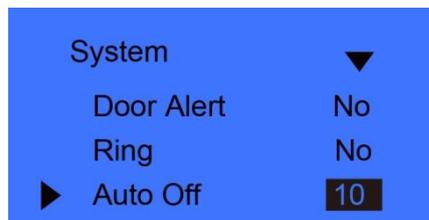
Press [◀ IN] or [OUT ▶] key or number key to input dormancy time. Press [OK] key to confirm. Then press [C] to save the setting.
