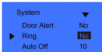
Press [◀ IN] or [OUT ▶] key or number key to input delay time value. Press [OK] key to confirm. Then press [C] to save the setting and press [OK] to be saved.
