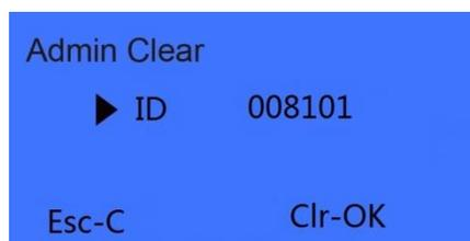
Press [OK] key to delete manager continuously. Press [C] key to exit manager clear interface as well.
