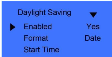
When you enable “Daylight Saving” function you need select week or date format first. Then you need set the time point for “Daylight Saving” start time and end time. And press [C] key enter save interface.
