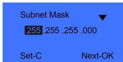
Press [◀ IN] or [OUT ▶] key or number key to input subnet mask. Press [OK] key to shift between the 4 segments. After set is completed, press [C] key to enter subnet mask save interface.
