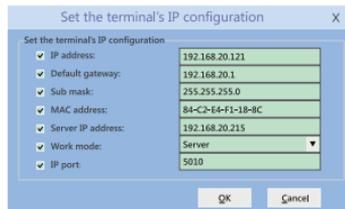
Right click on the device icon
