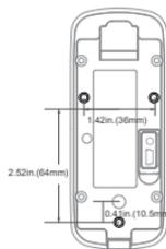
Behind the wall fix M4 screws directly to the bottom shell, the depth of screws is 8mm. This install method is unique, safe and convenient. Package list has no these screws, according to wall thickness select the length of M4 screws.
