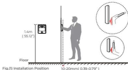
Fig.(1) Installation Position 10-20mm( 0.39-0.79" )
