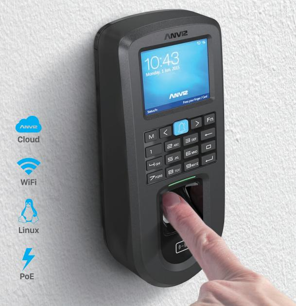
VF30 pro is the new generation standalone access control reader equipped with Linux based 1Ghz processor, 2.4" TFT LCD screen and flexible POE and WIFI communication. VF30 pro also supports webserver function ensuring easily self management and professional standalone access control interfaces. An standard EM card reader is also equipped onto the device.
